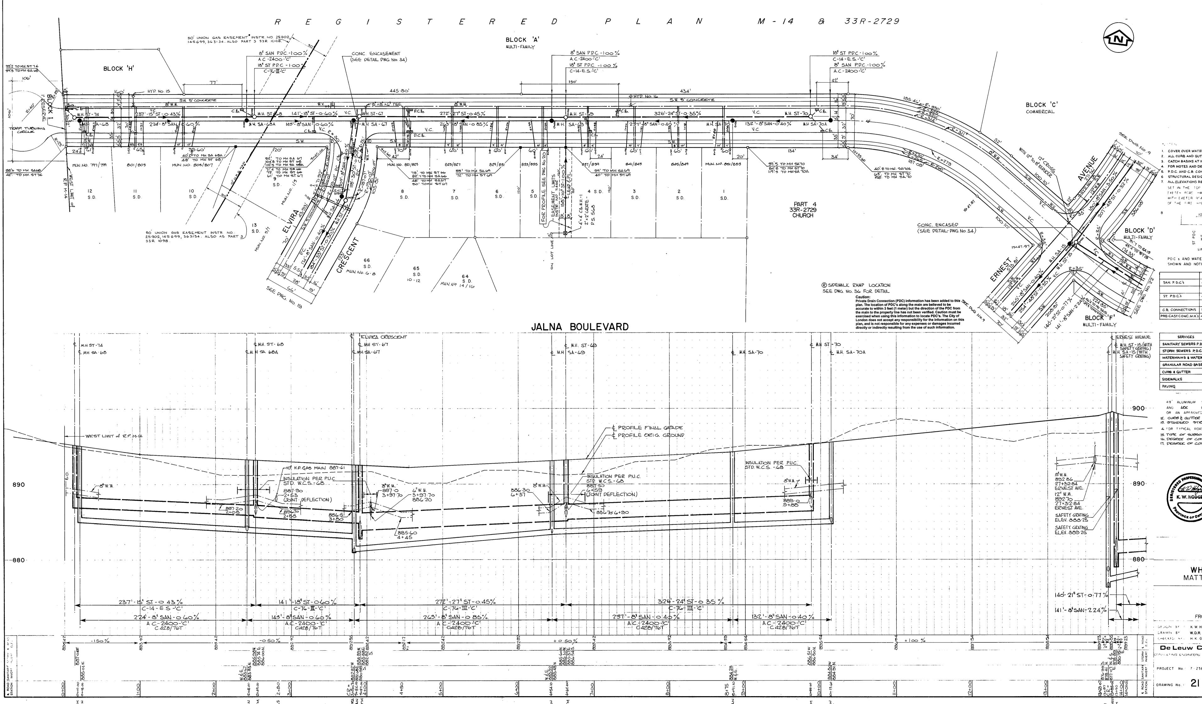
I. COVER OVER WATERMAIN TOP OF MAIN TO ROAD CENTRELINE IS 5-6 TO 6-0 UNLESS OTHERWISE NOTED. 2. ALL CURB AND GUTTER RADII 25 UNLESS OTHERWISE NOTED. 3. CATCH BASINS AT INTERSECTIONS ARE LOCATED 2 FT FROM B.H.C. OR E.H.C. CURVES UNLESS OTHERWISE SHOWN.
