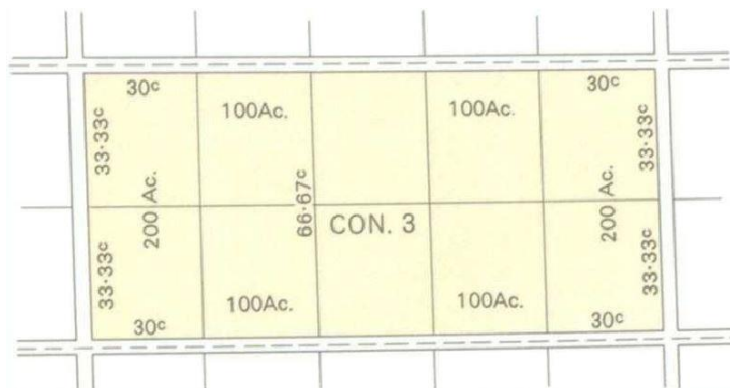
Plate 1: Double Front Survey System (Dean 1969)
