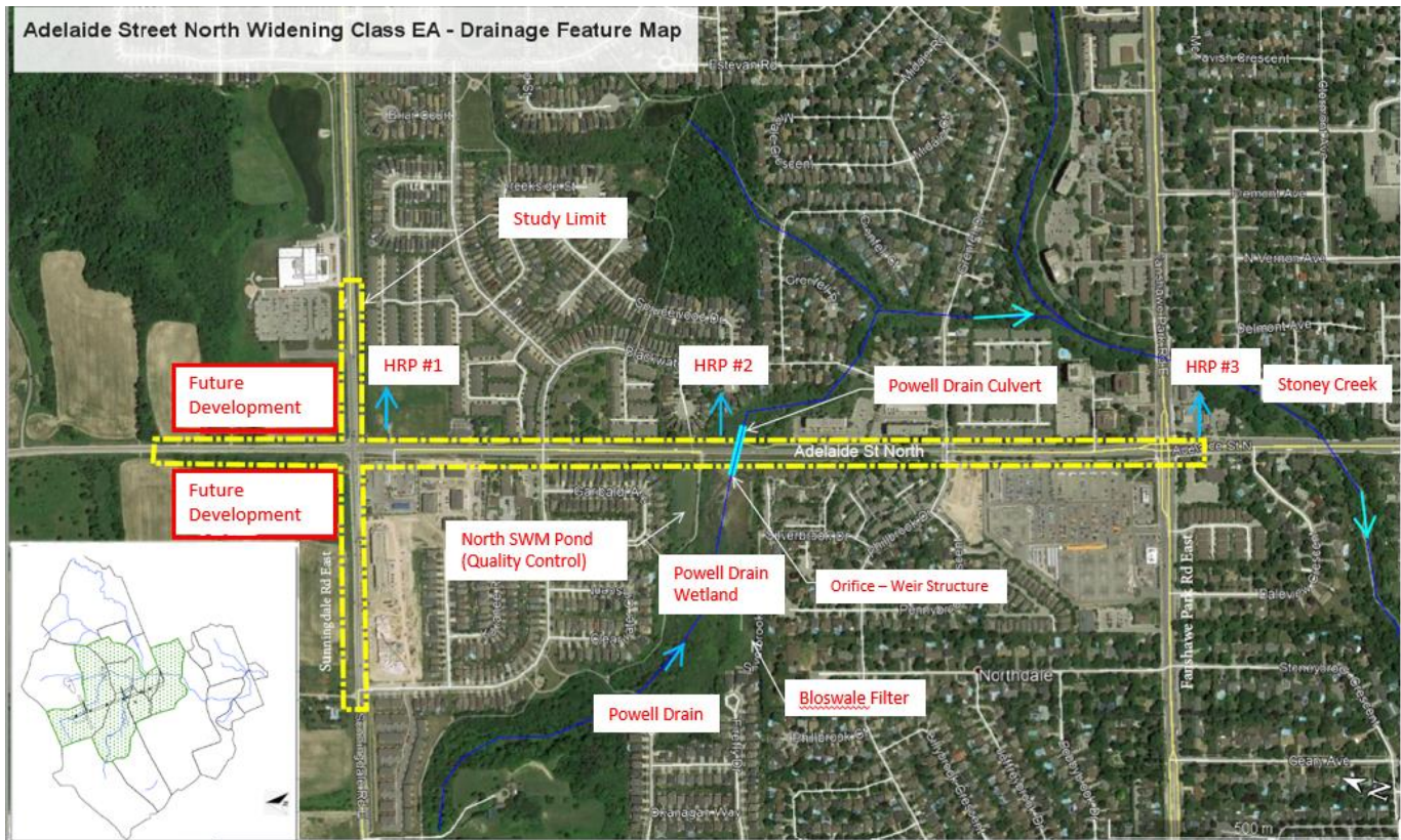
FIGURE 5: EXISTING DRAINAGE PATTERNS
