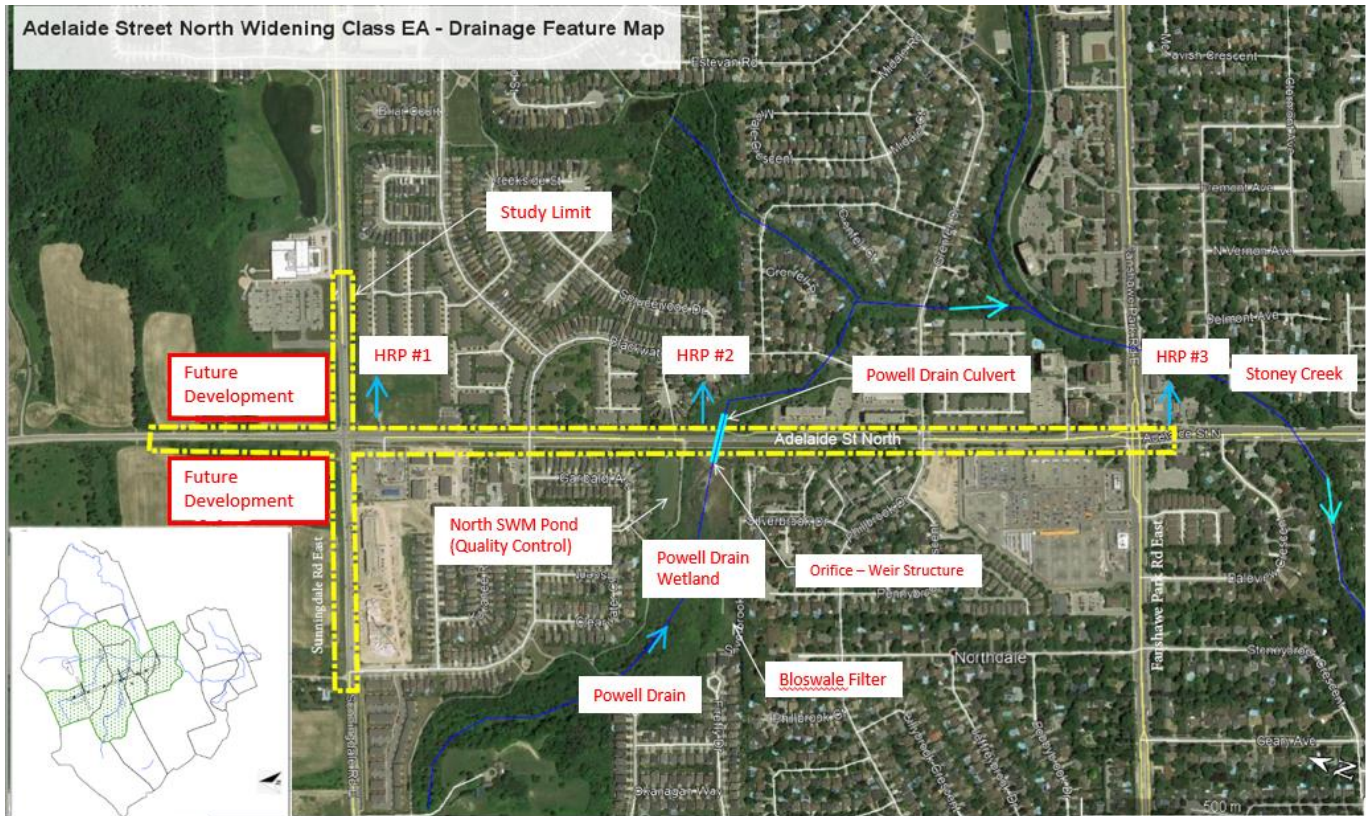
Figure 5 , the Powell Drain discharges the north-west segment tributary areas of the Stoney Creek watershed along the creek and crosses Adelaide Street North through a culvert. The Powell Drain wetland is located upstream of the culvert and an orifice-weir structure is installed immediately upstream of the culvert inlet headwall. The orifice-weir structure is designed and installed to provide a low flow regime in the creek and enhance the ecology of the wetland.
